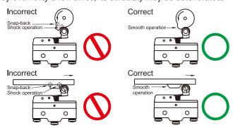
Make sure that no improper force is applied to the actuator, otherwise the actuator may incur local abrasion. As a result, the actuator may become damaged or its durability may be deteriorated.
