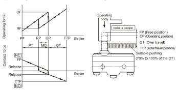
• Make sure that the operating body is set so that the actuator should return to the free position when the operating body has moved if a switch is used to form a normally closed (NC) circuit. If a switch is used to form a normally open (NO) circuit, the operating body must move the switch actuator to the distance of 70% to 100% of the rated over travel (OT) of the switch.
