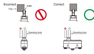
• Make sure that the operating body moves in a direction where the actuator moves. If the actuator is a pin plunger type, make sure that the operating body presses the pin plunger vertically.
